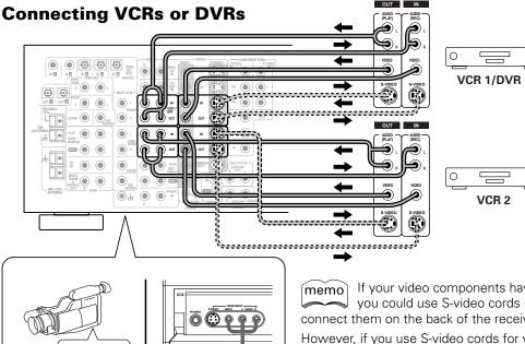
Front video connections are accessed via the front panel input selector as "VIDEO."
